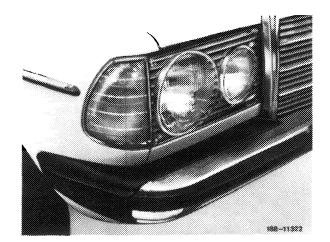
3 Unscrew screws in the headlight cutout, or the two sheet metal screws from below in case of the 2. version.
