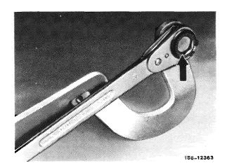
14 Force screw with a screw driver toward nut and tighten with hexagon ratchet.
