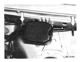
6 Pull hood cable control out of clips under radiator reinforcement.
