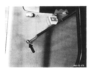
5 Pull cable control out of bracket on wheel house and loosen plastic tape.
