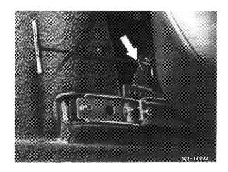
4 Unscrew screw at the slide rail and pull slide rail out of seat fitting.
