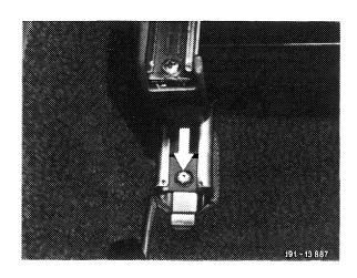
7 Remove screws from both front seat guide rails.
