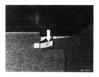
**Note:** The slide rail is inserted into the opening at the rest seat fitting and only mounted at the rear.
