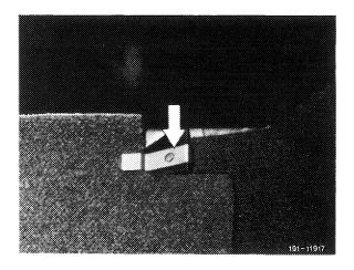
**Note:** The slide rail is inserted through opening on reclining seat fitting and is attached at the rear only.
