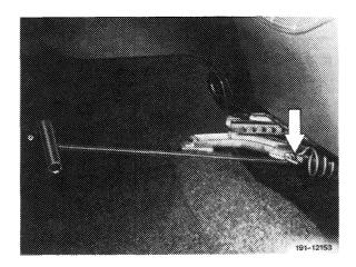
4 Remove screw on slide rail and pull slide rail out of seat fitting.
