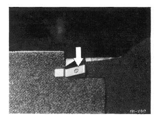
**Note:** The slide rail is inserted through opening on reclining seat fitting and is attached at the rear only.
