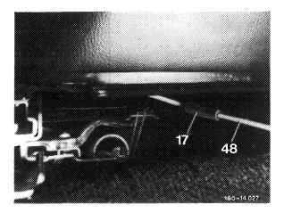
3 Drill out four hollow rivets (117) of the element retainer.
