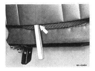
7 Pull out the three rivets on seat fitting.
