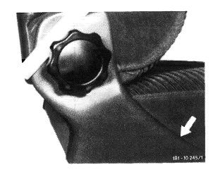
4 Remove screws on both sides of front seat cushion frame.
