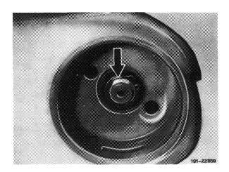
7 Remove buffer spring from bearing shaft.
