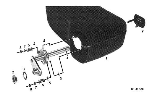
Bearing Washer Compression spring Washer
