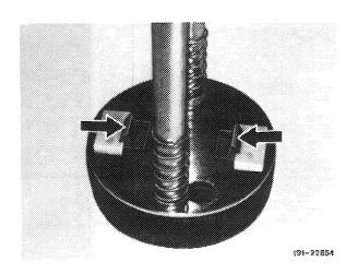
6 Remove locking ring from bearing shaft and pull out bearing shaft with bushing.
