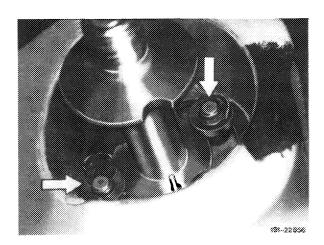
5 Remove actuating button with springs and disassemble, if required.
