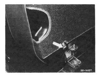
3 Push out cover at left and right adjacent to rear seat backrest by means of a plastic wedge.
