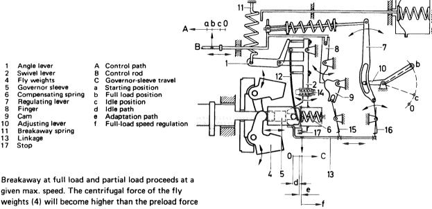
given max. speed. The centrifugal force of the fly weights (4) will become higher than the preload force of the breakaway spring (11), so that swivel lever (2) will move from housing stop (17) to the right.
