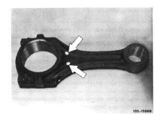
Connecting rods which are overheated as a result of bearing damage (blue discoloration) should no longer be used.
