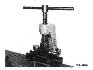
10 Check offset of connecting rod bearing bore in relation to connecting rod bushing bore and make corrections, if required.
