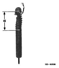
Rear shock absorber Boge a Length of exposed piston rod
