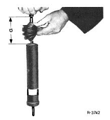
Rear shock absorber F & S up to October 1980 a Length of exposed piston rod
