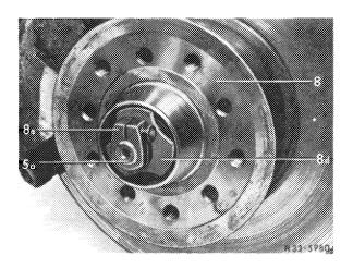
6 Place tester (015) on front wheel hub and set dial gauge (022) to approx. 2 mm preload.
