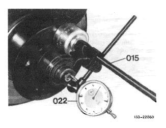
7 Check end play of wheel hub by pulling and pushing energetically on flange.
