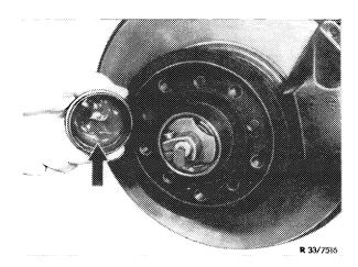
5 Loosen hex. socket screw of clamping nut (8e), then tighten clamping nut while simultaneously rotating hub (8) so that the hub can be rotated with an effort, only. Then screw clamping nut back again for approx. 1/3 turn and loosen tension by a blow against kingpin (5a) with a plastic hammer.
