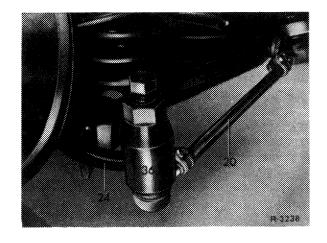
3 Unbend locking plate (21), unscrew hex. head screws (20) and remove steering knuckle arm (23).
