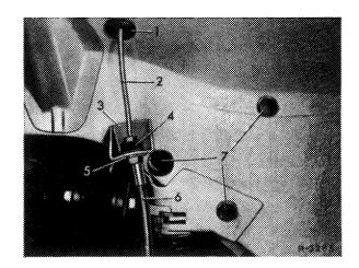
9 Check rubber sleeve (2) on ball pin of track rod. If rubber sleeve is damaged, renew ball joint (46–540). Fasten track rod to steering knuckle arm. Tightening torque of castle nut 35 Nm reference value. Cotter castle nut.
