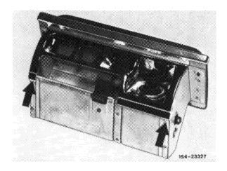
3 Slightly pull out ashtray top under covering strip and remove in upward direction.
