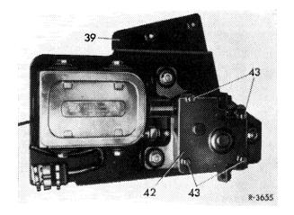
4 Remove gear unit cover (42) and take off large gear wheel (44) including drive shaft (45).
