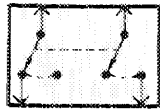
SWITCHES THAT MOVE TOGETHER DASHED LINE SHOWS A MECHANICAL CONNECTION BETWEEN SWITCHES
