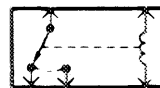
RELAY SHOWN WITH NO CURRENT FLOWING THROUGH COIL WHEN COIL IS ENERGIZED, SWITCH IS PULLED CLOSED
