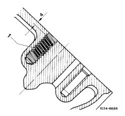
10 Screw a cylinder head bolt into the inserted thread and check for misalignment and easy operation.
