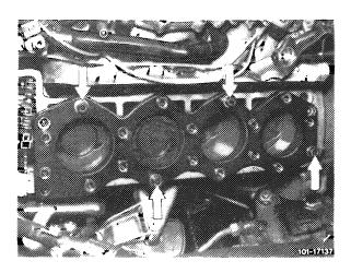
3 Using an HSS spiral drill 10 mm dia., drill core hole approx. 37 mm deep while lubricating with honing oil.
