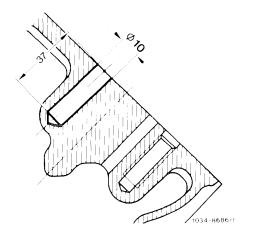
4 Remove drilling jig and blow out chips.
