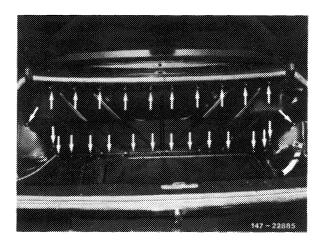
5 On vehicles with battery in trunk, remove battery and battery casing (arrows).
