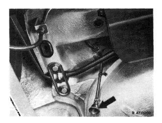
7 On vehicles in (a)-, (J)-, and (usa) version, pull fuel hose (arrow) from vent line.
