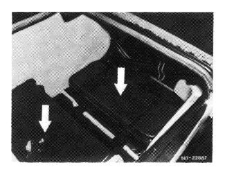
6 Remove protective sleeve (arrow) and pull vent line out of holding clamp.
