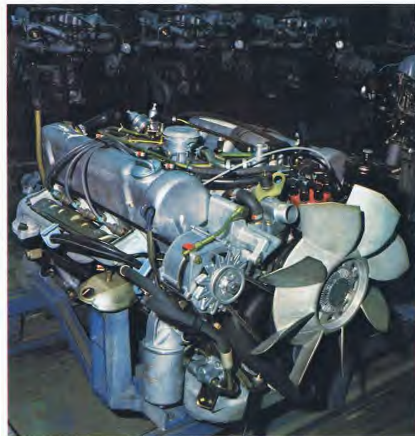
3.5 litre V-8 engine with electronically controlled petrol injection. Transistorized ignition and visco-drive fan dependent on the engine speed.
