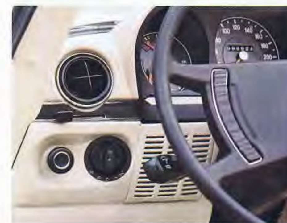
Mercedes-Benz do not believe in an imposing array of switches and showy interior fittings. Non-dazzle materials are better than visual opulence. Flush-fitted switches and buttons are additional safety factors.
