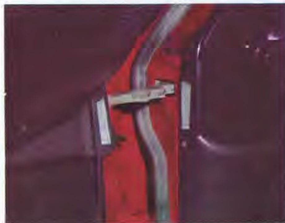
An air duct connects the doors of the 350 SL to the heating and ventilation system.
