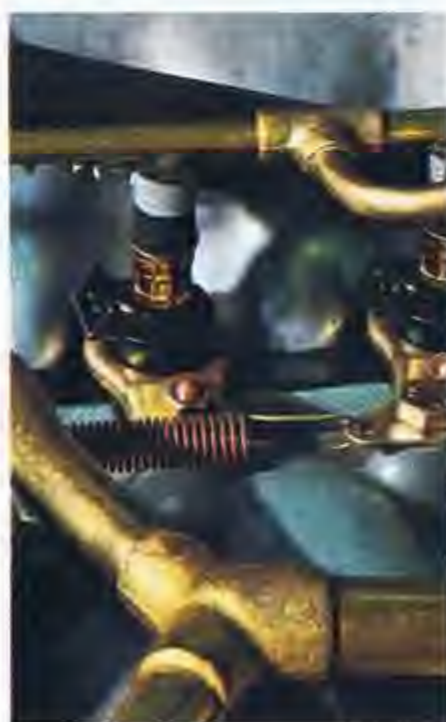
3.5 litre V-8 engine with electronically controlled petrol injection. Transistorized ignition and visco-drive fan dependent on the engine speed.
