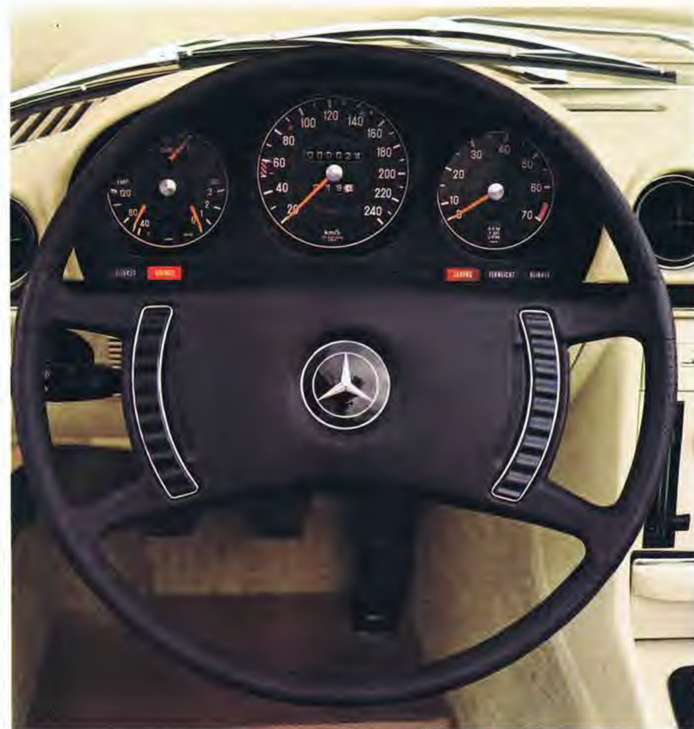
The four-spoke safety steering wheel. The padded boss, spokes and rim form one foam-padded unit.
