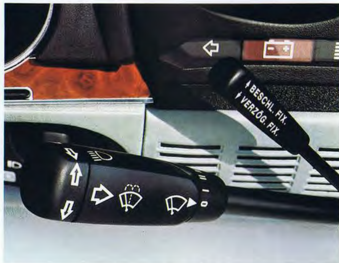
The combination switch, which operates the low-beam headlights, the headlight flasher, the indicators, the windscreen wipers and the screen wash system.
