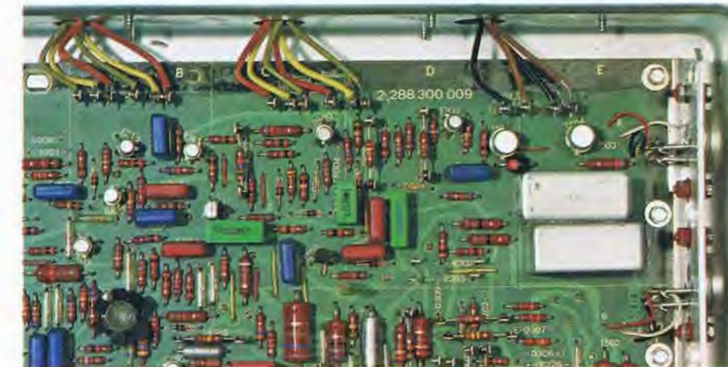
In a split second the electronic control unit determines the correct amount of fuel, according to the speed and operating condition of the engine.
